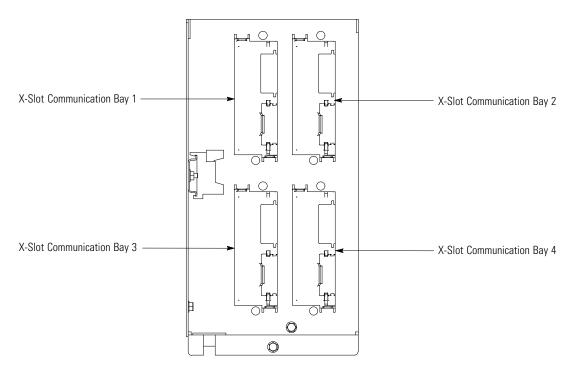
Figure 4-33. X-Slot Communication Bays
